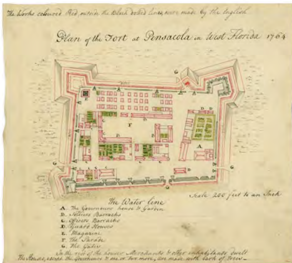
Plan of the British fort at Pensacola, 1764. (Image courtesy of the Brown University Library)
