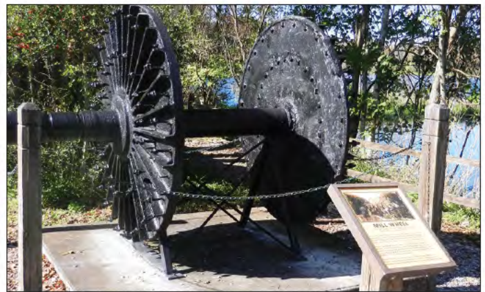
Waterwheel hub and axle, De Leon Springs State Park.
