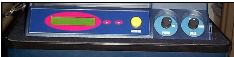
Figure 1 Backside of the AVC EDGE DRE with activation button, power switch, and poll switch
