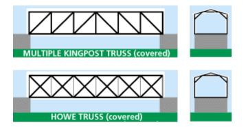
Stephen H. Long (1784-1864) was one of the U.S. Army Topographical Engineers sent to explore and map the United States as it expanded westward. While working for the Baltimore and Ohio Railroad, he developed the X truss in 1830 with further improvements patented in 1835 and 1837. The wooden truss was also known as the **Long truss** and he is cited as the first American to use mathematical calculations in truss design.
