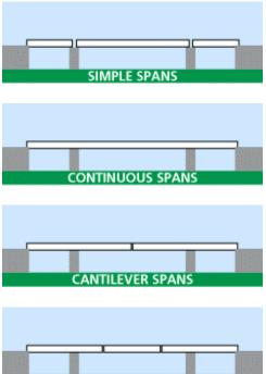
CANTILEVER SPANS (with suspended span)
